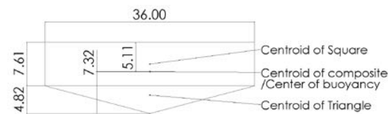
Figure 5 - Waterline at Center of Gravity Front View
