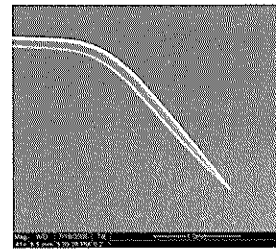
Figure 13: Experimental probe exposed to single spot bending with a bend angle of 135
