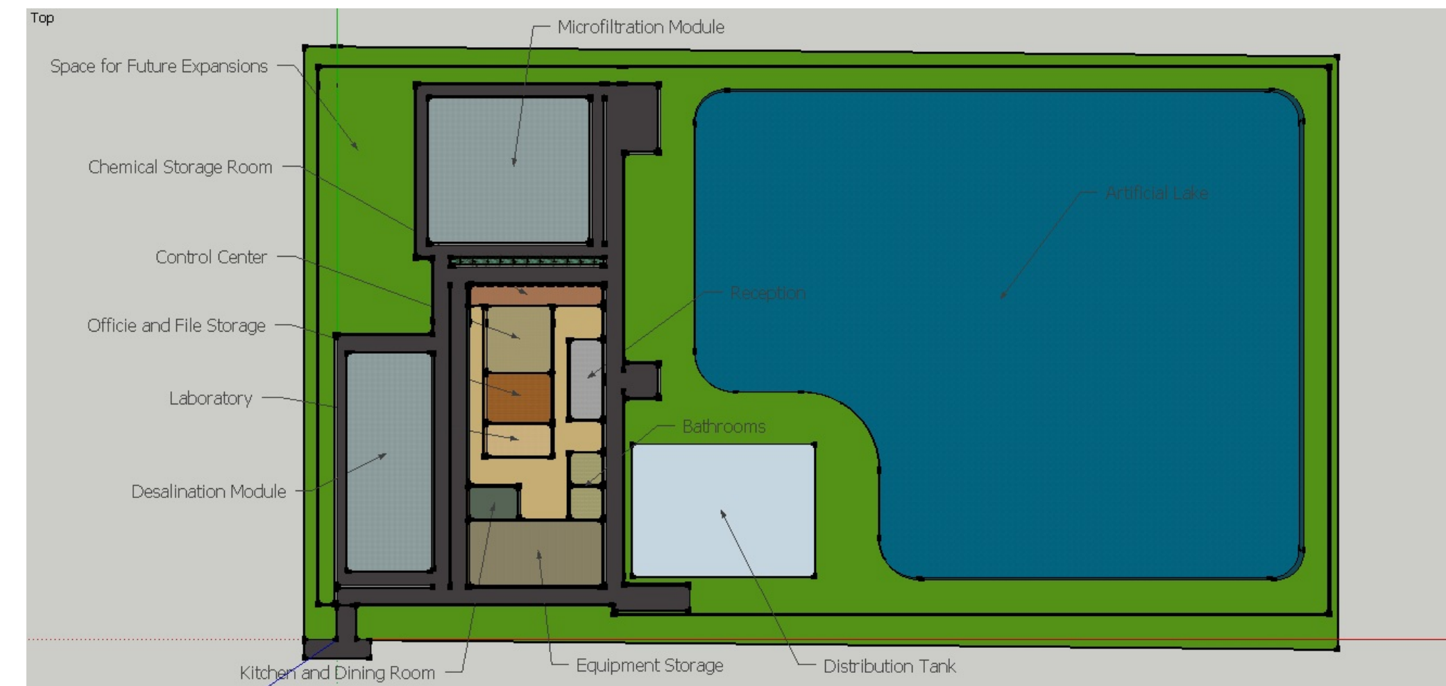
Image 2, 3 & 4: Water Desalination Plant Layout and Connections
