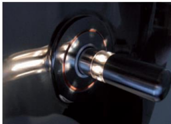
Figure 1 GEA Pharma Systems LHP-A-2”SP Probe Installed in Process Equipment
