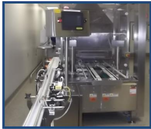
Figure 1 Crimp Quality Automated Inspection System
