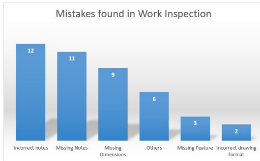
Figure 5 [6] Mistakes Found in Work Inspection
