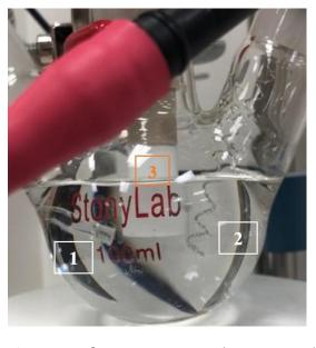
1. Reference Electrode 2. Counter Electrode 3. Working Electrode
