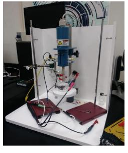
Three-electrode cell set-up
