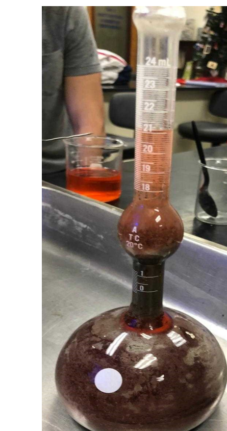
Pycnometer test for cement.
