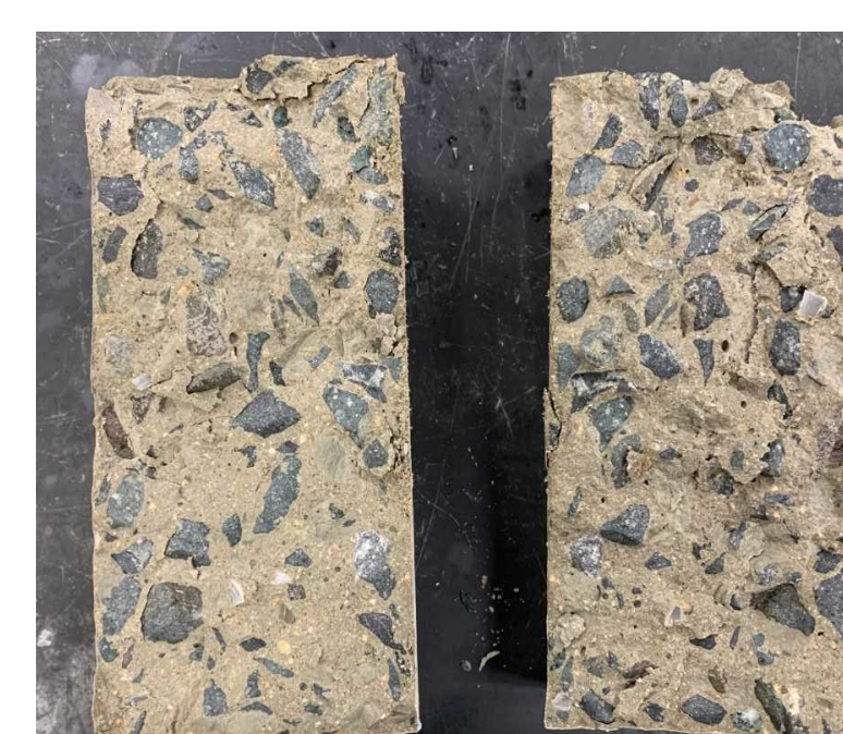
Split (tension) test (ft) at 28 days, 2 cylinders per admixture (14 total tests).
