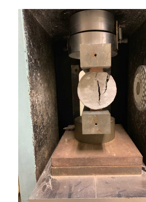
Split (tension) test (ft) at 28 days, 2 cylinders per admixture (14 total tests).
