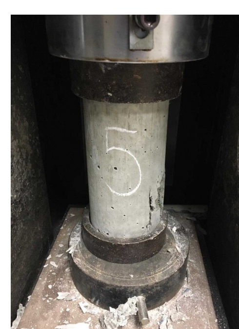
Compression test, 84 total compression tests.
