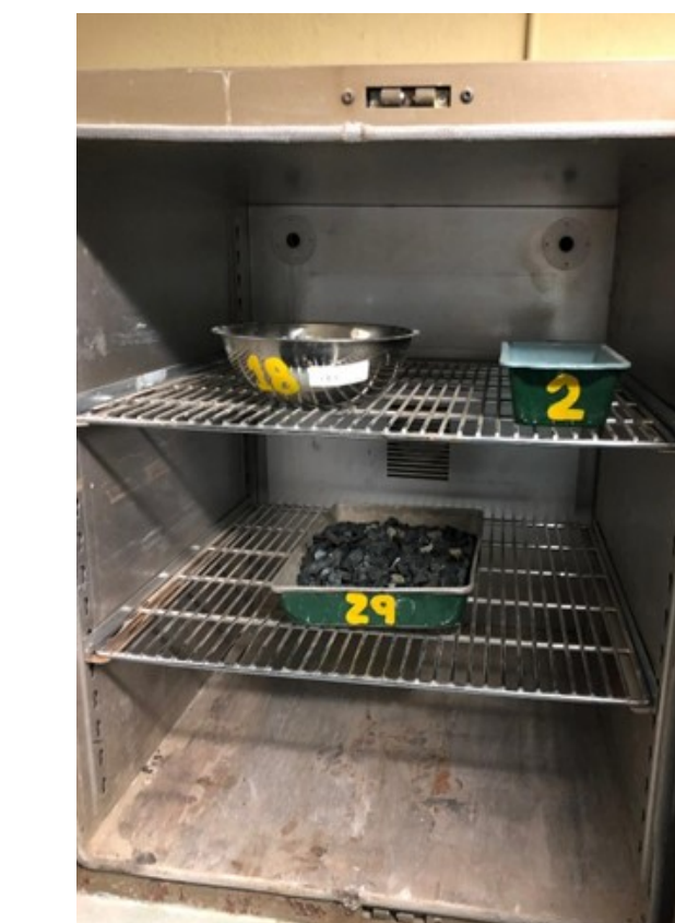
Moisture content for fine and coarse aggregates.
