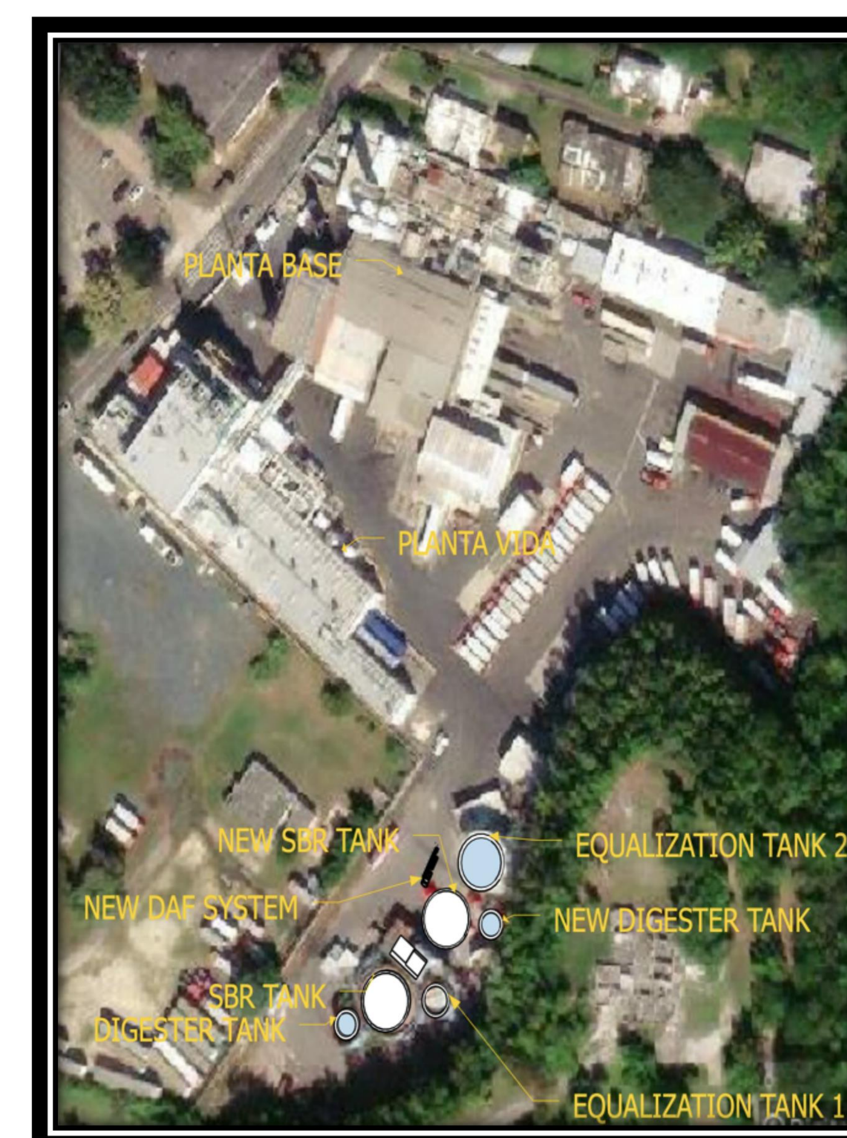
Figure 3 Diagram after Improvements of Water Treatment Plant
