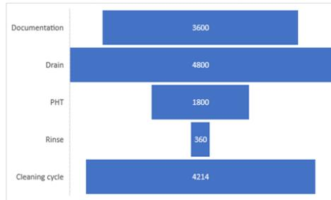
The data included in the figure above have the consumption time of each stage. If the chart was studied, many stages are repetitive. The total time of each stage were evaluated and consolidated in the project to reduce the cycle time of the cleaning recipe. Each stage was consulted with the validation personnel to determine the critical step of the recipe and they confirmed that no step can be eliminated, but can be consolidated.
