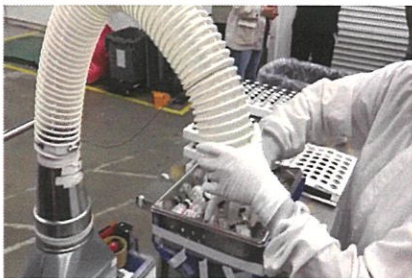
Figure 4 - Cleaning of Vials using Blown Air
