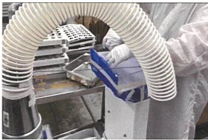
Figure 2 - Placement of Filter for Particle Collection
