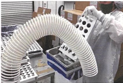
Figure 3 - Unloading of Vials into Stainless-steel Bin
