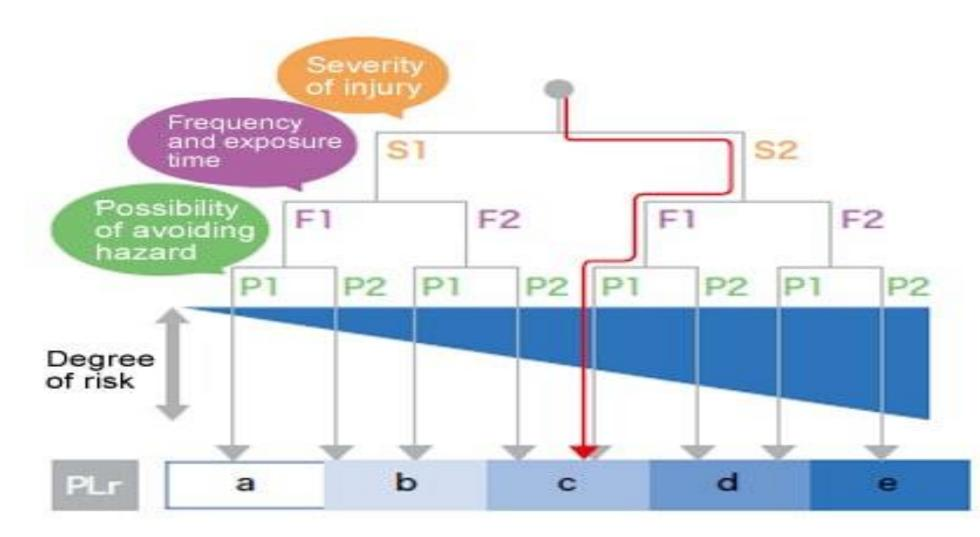
Relationship between the performance level (PL) of safety related parts on a control system, supposed to be equal or higher than the required performance level (PLr).
