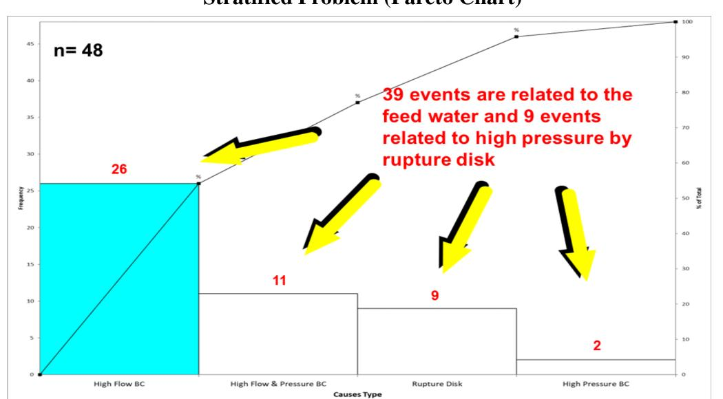
The Pareto Chart shows the frequency of events per group, confirming that 39 events were caused by the feed water fluctuations. The remaining 9 events were caused by a pressure backup from the degasifiers. Based on these findings, the problem statement was defined as "Permeate water overproduction, and high pressures can create scaling when particles accumulate on a membrane, causing the membrane's pores to plug."
