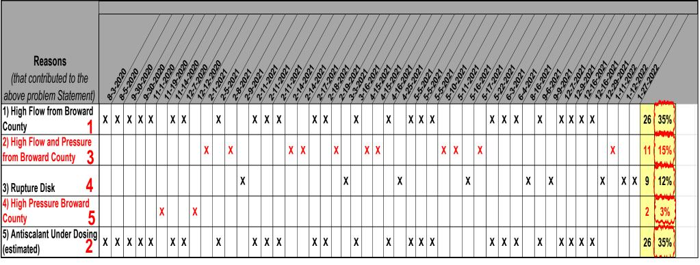
The single case bore analysis used the four groups of data obtained in the measure step. The SMEs added an additional reason: "Antiscalant underdosing," considering that a sudden increase in feed water flow can cause the antiscalant injection system to under-dose. The reasons were validated per period, adding the frequencies for each one, and then dividing them by the total of occurrences to obtain a percentage of occurrences.
