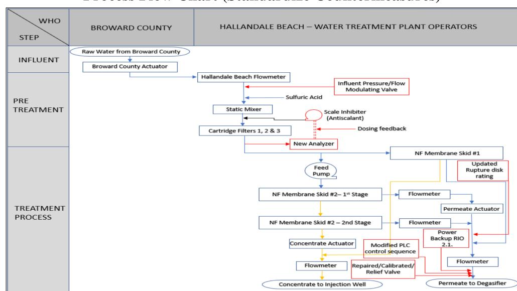
The countermeasures were integrated into the process flowchart, with the exact location of each one in the process.
