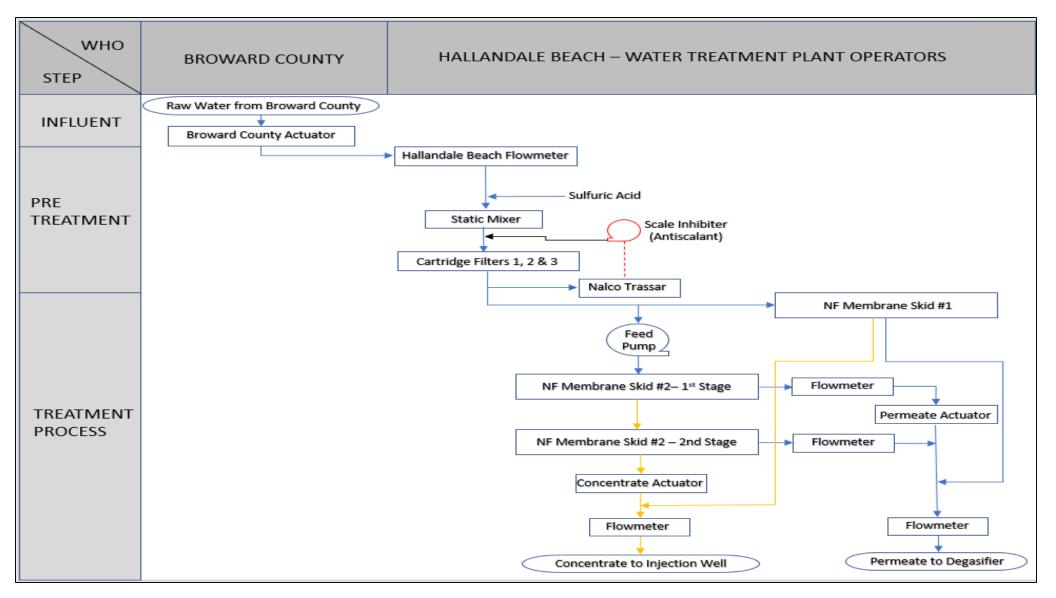
The Process Flow Chart describes the different components and elements that are part of the process, who are responsible for each operation, and the overall phases in the treatment (influent, pre-treatment, water treatment).
