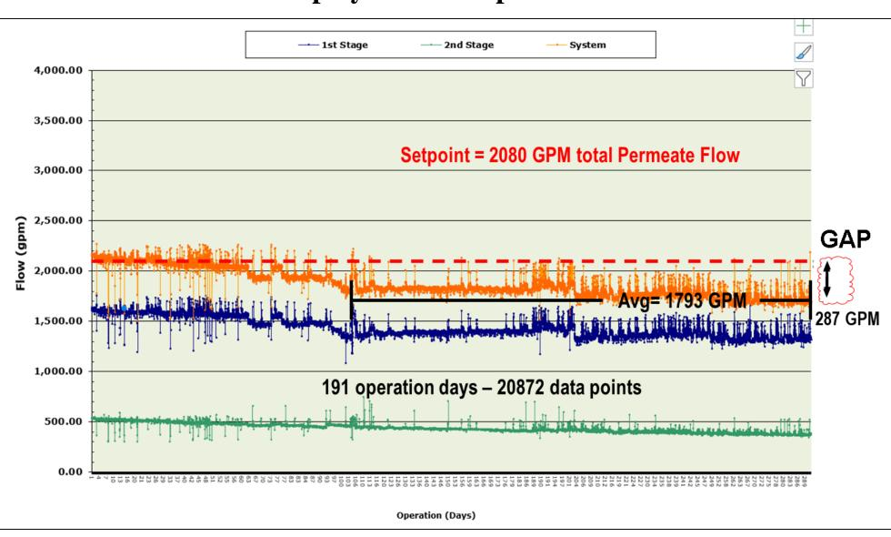
As shown in the Display Indicator Performance figure, the permeate flows decreased from the established setpoint of 2080 gallons per minute (gpm) until an average of 1973 gallons per minute (gpm).
