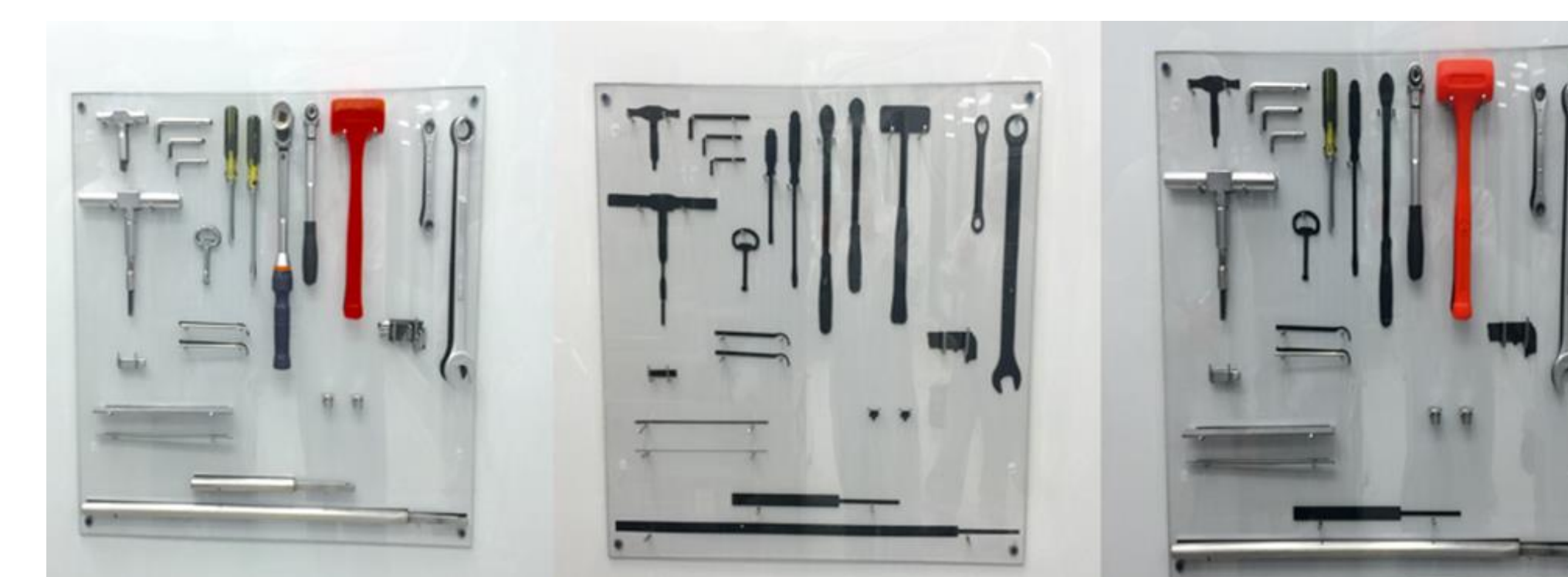
Figure 2 In-Process Shadow Boards Installation
