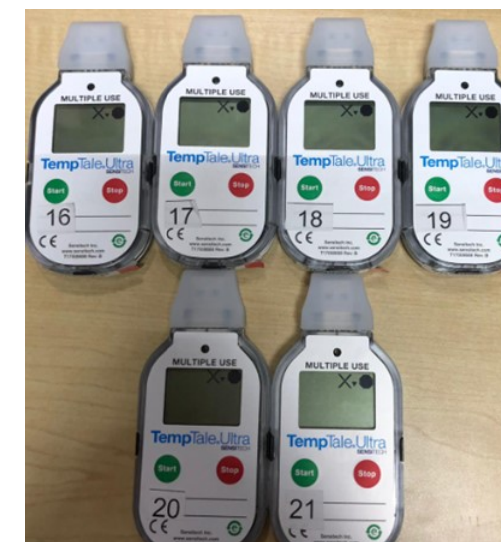
Figure 3 TempTale®Ultra sensors in where the temperature excursions were found. Sensors B3S16, B3S17, B3S18, B3S19, B3S20, and B3S21 were identify with the temperature excursions, as showed on Figure 3.
