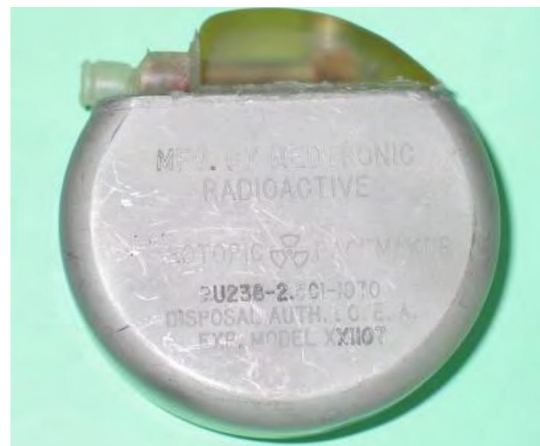
Figure 8 Pacemaker Using a Nuclear Battery
