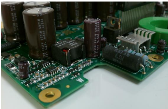
Figure 1 Surface Mounted and Plated Through-holes Components
