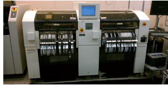
Figure 3 Panasonic CM202 Pick and Place Machine
