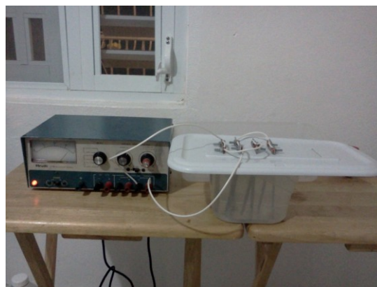
Figure 2 Electrocoagulation Cell with Aluminum Electrodes
