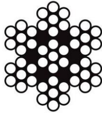
Figure 4 7x7 Wire Rope Cross Section
