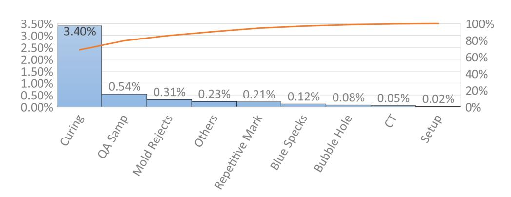
After understanding that curing was the biggest offender, we focused on what is curing losses. It defined as all the molds that arrived in the bags as final products after the curing oven, divided by all the molds picked up by the CUA (Control Unit Acquisition).
