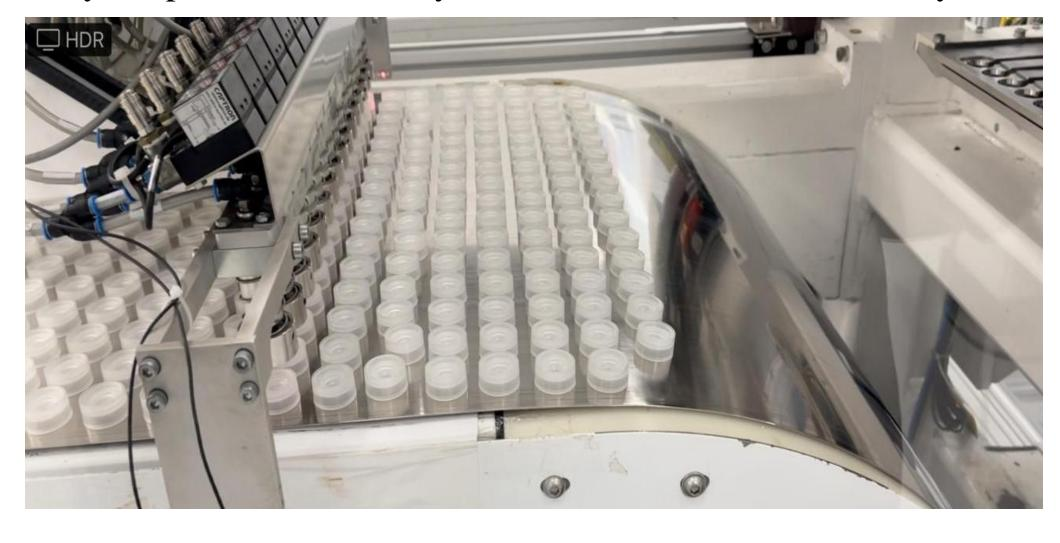
On top of the steel conveyor, we have the CUA (Control Unit Acquisition). This is the one in charge pciking up the molds from the steel conveyor and delivering them into the walking beam. This is where the machine start to consider molds as good and if discarded after it would impact the yield as curing losses.
