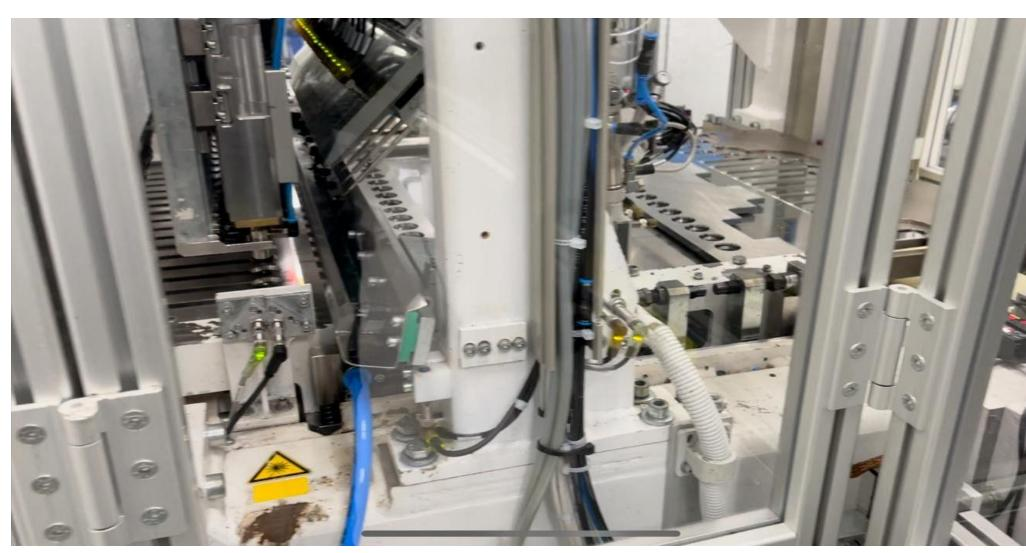
If the molds was good, it would then be transferred to the loading conveyors, each oven have its own loading conveyor. The loading robots are servo controlled and pick up the molds in the walking beam and loads them into the conveyor.
