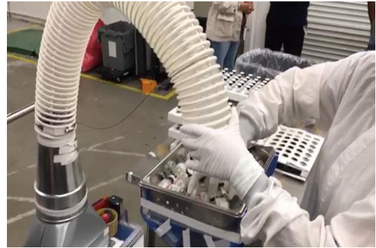
Figure 4 Cleaning of Vials using Blown Air
