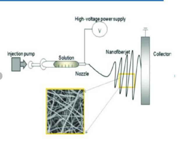
Electrospinning is considered one of the most common technologies to produce nanofibers; and the basic machine setup for operation comprises a nozzle connected to a high-voltage DC power supply, a grounded collector and a solution reservoir to supply polymer solution [2].
