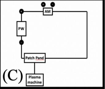
[Fig 3 (c)] DC Circuit of the electrostatic plasma with an amperemeter, power supply connected to a patch band
