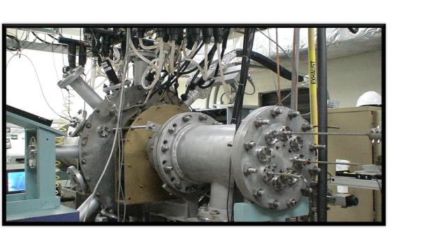
[Fig 2] Electron Cyclotron Resonance Plasma (ECRP) and Eletrostatic Plasma camera -Plasma laboratory at PUPR - machine were bacteria sterilization trials were placed.
