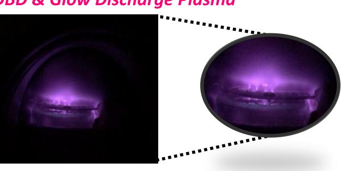
[Fig 3 (e)] Dielectric Barrier Discharge Plasma trial at PUPR Plasma Laboratory 05.15.2019. Showing direct glow through the Corning Petri dish.
