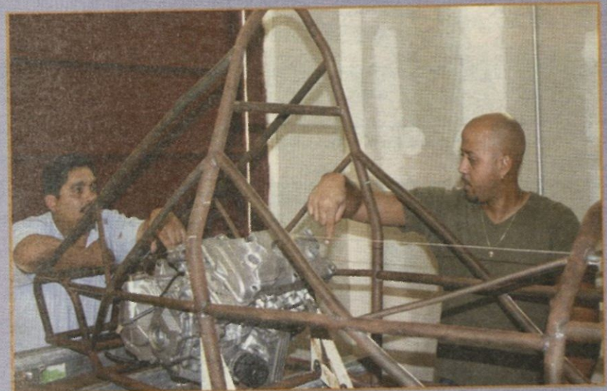
Students locating the engine within the frame of the Poly Formula Car
