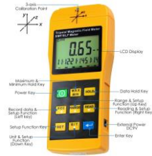
Figure 2: Gauss Meter Measures Direction and Intensity of Magnetic Field
