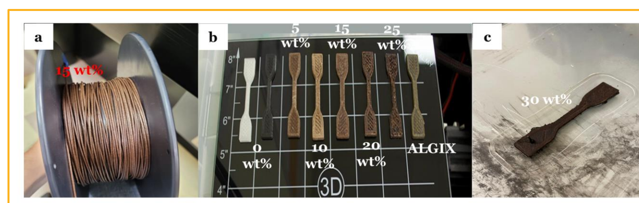
Figure 11. Images of (a) a fabricated filament, (b) and (c) different dog-bone-shaped specimens for the tensile tests.
