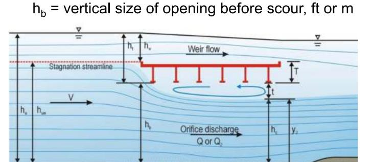
Local scour is calculated independently for abutments and piers. HEC-18 provides various equations to estimate scour at abutments, including the Froehlich Eq. and NCHRP 24-20 Eq., which estimates total scour rather than local scour only.
