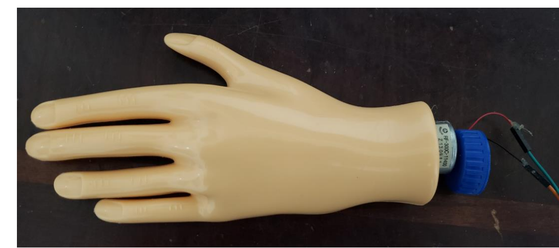
Figure 1: PD simulation of the hand tremor
