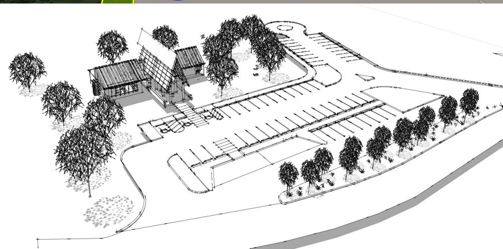
The impact area consists of 1 Acre, providing 60 parking spaces, of which 5% are for handicaps and 3% are for low emission vehicles. Considering collective transportation, the parking has two spaces for buses equal to 25 feet or less. The parking lot design considered a traffic study performed to calculate the National Forest vehicular demand. The three structures were designed with a combination of steel and concrete.
