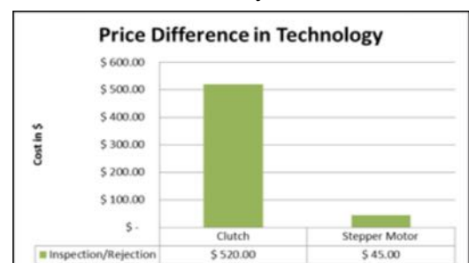
Figure 12 - Clutch vs. Stepper Motor Costs
