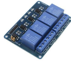
Figure 7 4-channel Relay used in the Design
