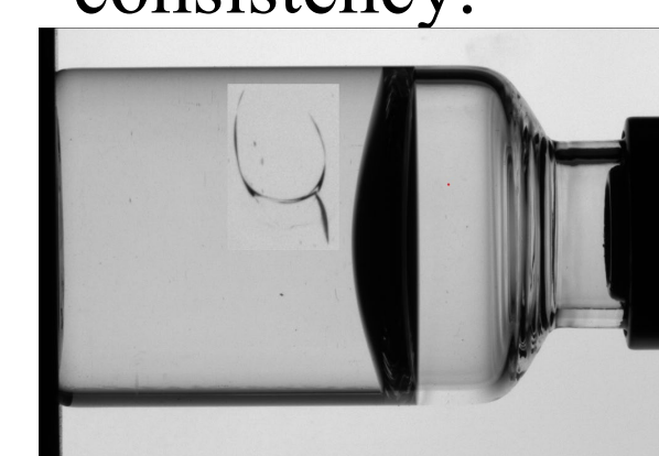
Figure 4: Crack defect insertion using Copy and Paste
