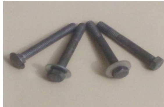
Figure 5 Bolt and Washers Used in the Laboratory Test
