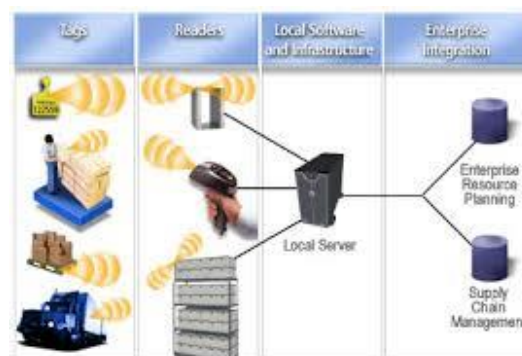
Figure 7 Functionality of Radio Frequency Identification (RFID)
