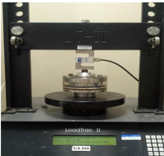
Figure 6 Geocomp Load Trac II Equipment
