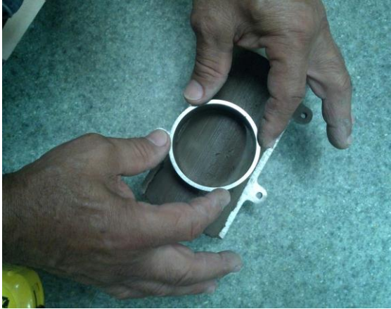
Figure 2 Example of Cutting Sample for Consolidation with Allowing Radial Drainage
