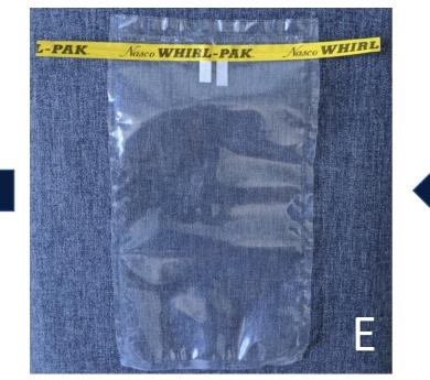
[Fig 5 (E)] Sterile bags for transportion of biological material. Used to transport bacteria from laboratories to avoid external contamination of samples.
