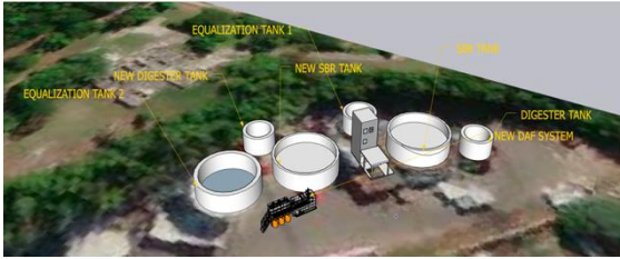
Figure 2 Diagram after Improvements of Water Treatment Plant
