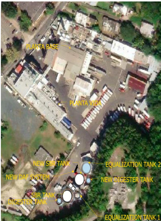
Figure 3 Diagram after Improvements of Water Treatment Plant
