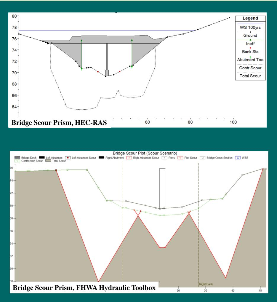
From these figures it can be observed that even though they present the same behavior, it was demonstrated that the scour values can be differentiated up to 50% like the scour depth for the right abutment, especially if the equations applied in each model were different, as in this case.
