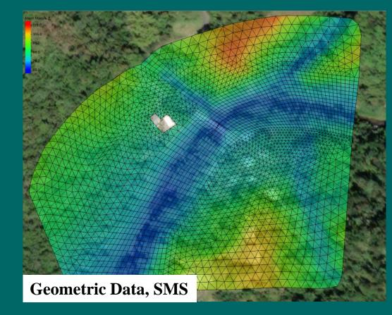
The topographic information used in the 2D simulation is the product of a merge between the ground elevation points took by the land surveyor and points from a U.S. Geological Survey LiDAR DEM from 2018. With this information and the surface's roughness information the mesh for the 2D model was completed.
