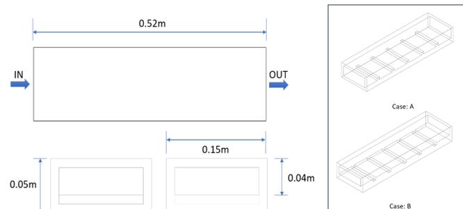
Figure 4. Dimensions of the Cooling Channel (Dimensions are in Meters)
