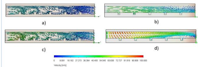
Figure 7. Velocity Distribution along the Cooling Channels at Re=5,000 for Case A), Case B) and Re=10,000 at Case C), Case D)
