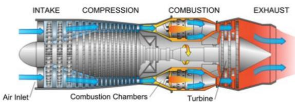
Figure 1. Gas Turbine Engine
