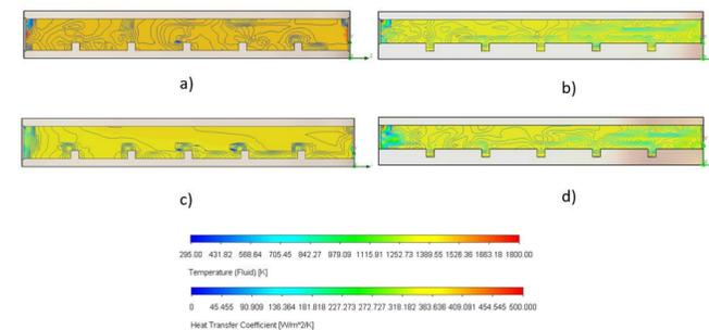
Figure 6. Temperature and Heat Transfer Coefficient Distribution along the Cooling Channels at Re=5,000 for Case A), Case B) and Re=10,000 at Case C), Case D)
