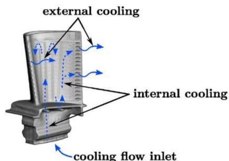
Figure 2. Gas Turbine Internal Cooling Passage
