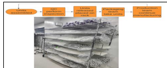
Figure 2 Dilator Current Replenishment Process
