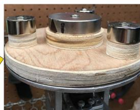
Four magnets hold the robot's head on the sphere, while a servo motor drives the head's movement from side to side.
