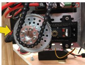
A servo motor drives the robot's turning by tilting the pendulum left and right.
