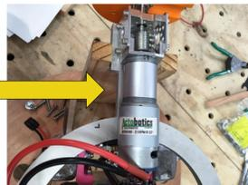
Two drive motors, located at the center of the sphere drive the robot's displacement by moving the pendulum forward.
