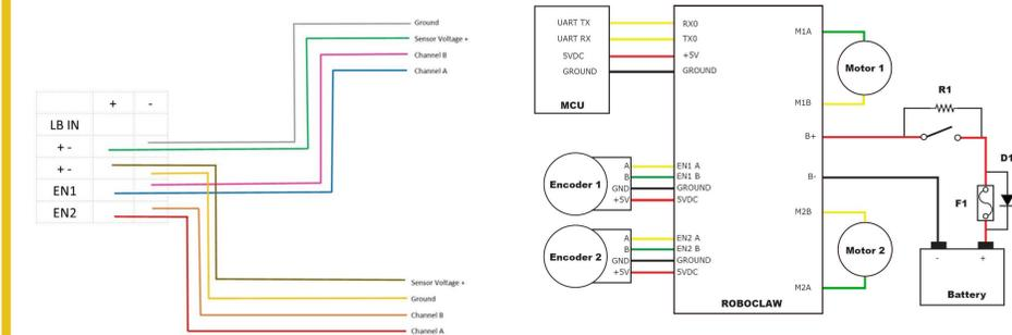
Wire color diagram between the motor controller and encoders
