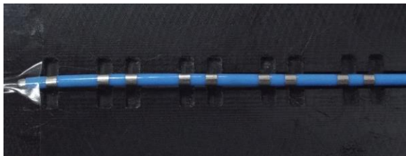
Figure 10 Catheter with Band Spacing Incorrect Defect using current template
