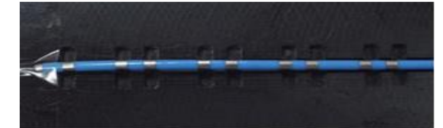
Figure 10 Catheter with Band Spacing Incorrect Defect using current template
