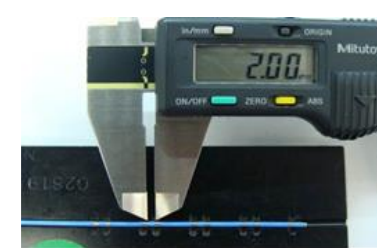
Figure 9 Verification with Caliper
