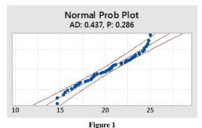
Normality Test for Size 2 USP Needle Pull Data
