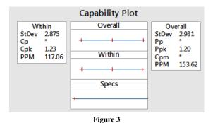
Process Capability Analysis Results for Size 2 USP Needle Pull Data
