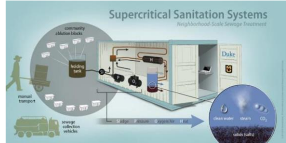
Figure 6 Supercritical Sanitation System Prototype
