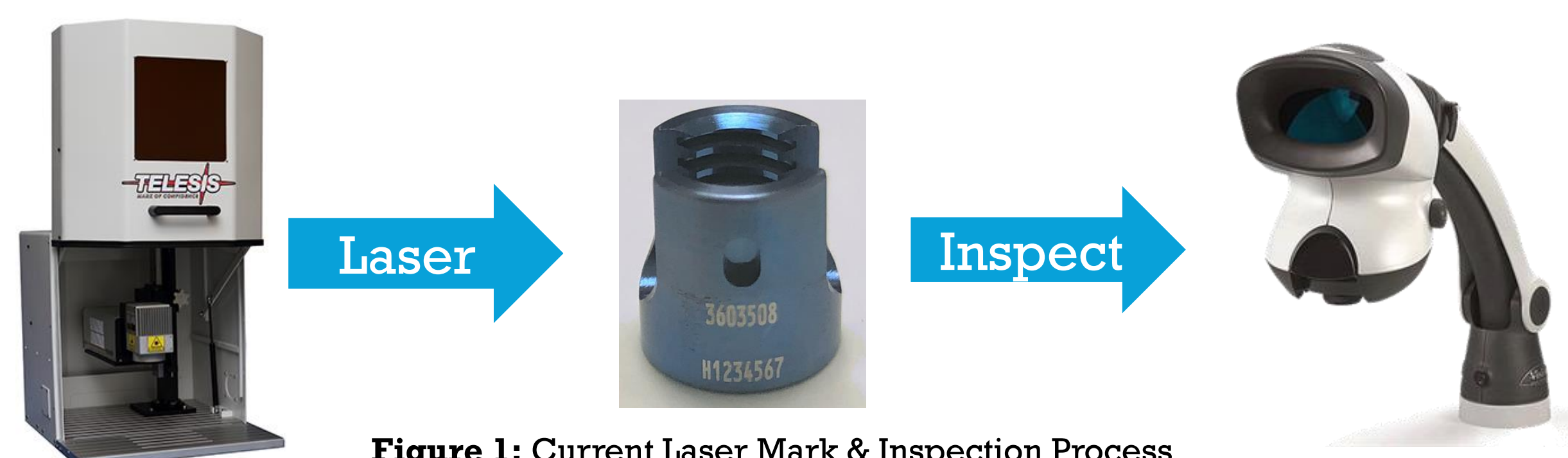
Figure 1: Current Laser Mark & Inspection Process
