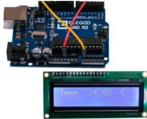
Figure 8 Temperature Monitor Design
