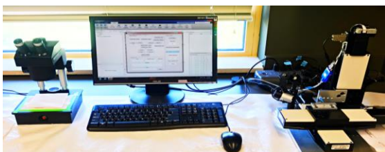
Figure 8 Micro-precision Coating Equipment with Microneedles
