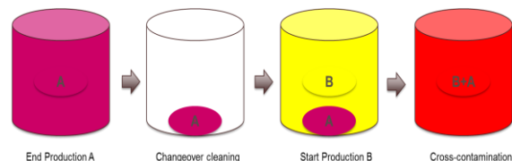
Figure 1 Risk-of-Cross Contamination caused by Poor Cleaning Design
