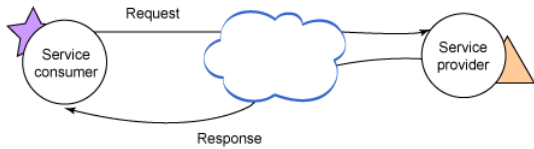
Figure 2 The Request/reply Mechanism in a SOA
